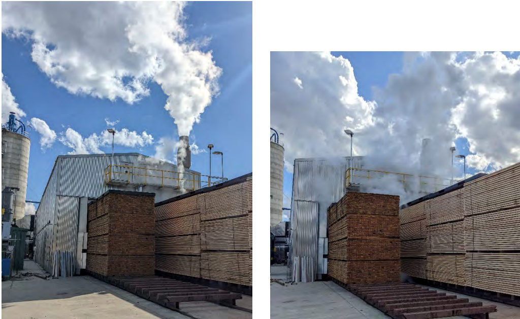
Figure 2. Side-by-Side Comparison of a CDK with its VEM On (Left) vs Off (Right)
